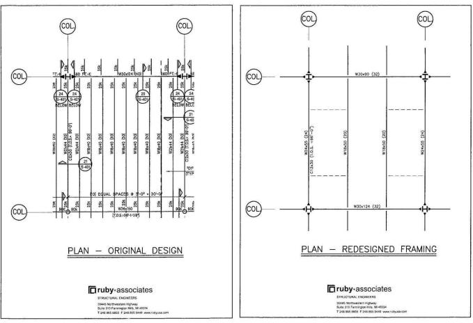
By applying constructability to this project, the team maintained design intent and made the project easier to build. Seven hundred steel members and 1,400 connections were eliminated, while shear studs were reduced by 11,000. Overall, approximately 300 tons of steel were saved.
